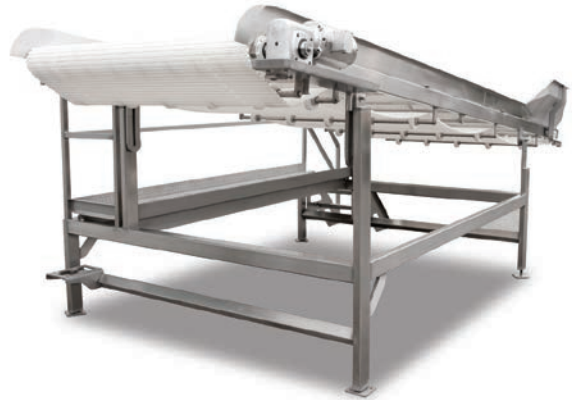
This slightly inclined conveyor transfers raw leaf products from a sorter and dumps the product into the first of a series of large wash tanks. The 5' wide x 15' long conveyor operates at 180 ft. per minute and is routinely subjected to high-pressure washdowns. A Boston Gear Stainless Steel 700 Series speed reducer was mounted to a stainless steel motor to meet the requirements of this challenging environment.
