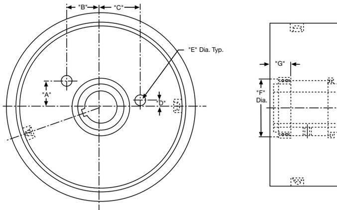
**Figure 8 - Type "B" Housing Configuration**
